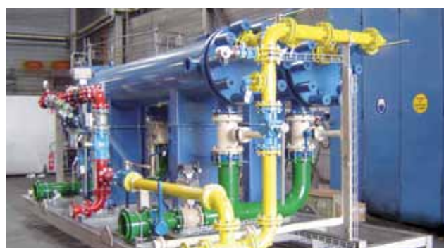
Sulfuric Dilution Unit. 86 333 kg/h 84% H 2 SO 4
